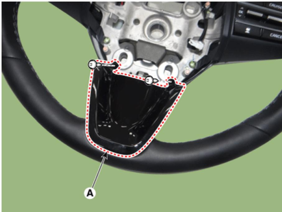
6. Remove the steering rear cover (A) after loosening the mounting screws.
