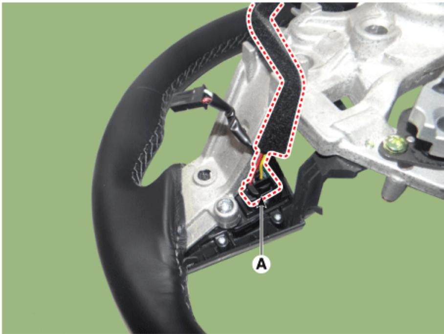
9. Remove the steering wheel remote control (A) after loosening the mounting screws.
