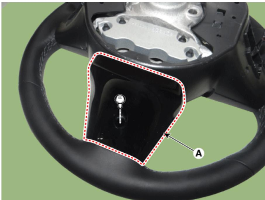
7. Remove the steering back cover (A) after loosening the mounting screws.
